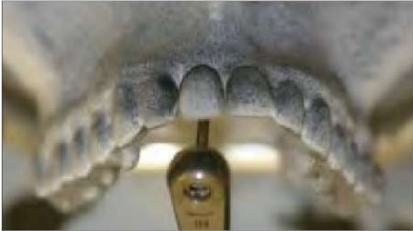
Fig 3 A random dot pattern is applied to the cast and the crown during tightening with a torque wrench.
