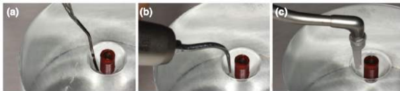
FIGURE 2 Engineering drawings of the three different defect models (a) 30°, (b) 60°, and (c) 90° each with an exemplary inserted photograph of an untreated implant (Replace Select Straight, Nobel Biocare AB, Göteborg, Sweden) 13 x 4.3 mm with 1.5 mm collar-height and 0.6 mm thread-distance
